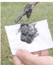
Coal Tar sludge was so thick and sticky, a sizable sample could easily be collected from the drain.
