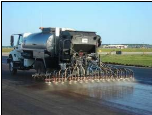
Figure 24. Distribution truck with acceptable sanding equipment.
