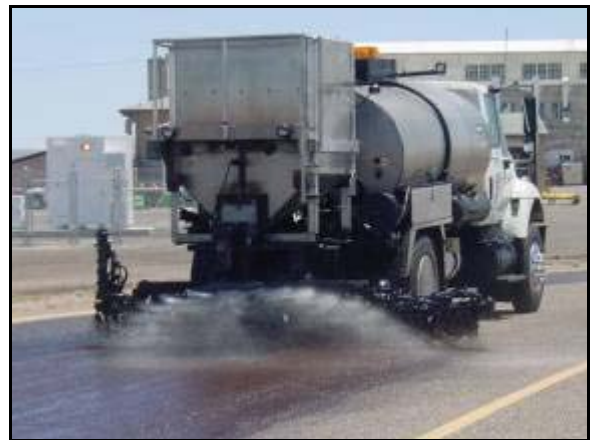
Figure 25. Distribution truck with acceptable sanding equipment.
